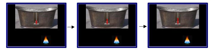
So let's set it on mark 2 and watch the temperature, there we go and you see the temperature starts to go up and up and up. It eventually reaches a point where the energy coming in from the burner balances the extra energy going out into the environment because the whole bath is a bit warmer. And if you want it warmer than that you have to turn the burner up higher. Good simulator. Not complex. Not even complicated. Just simple.
