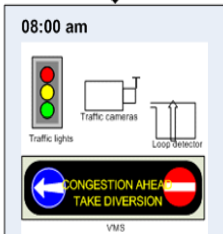
ITS system that monitors real time traffic conditions
